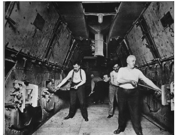
Firemen on the Hudson River Day Line steamer, Washington Irving shovel coal into the fireboxes
