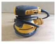
**Design Function:** The pad sander is a finishing tool. It is designed to smooth the surface of the wood and prepare it for a finish. It should not be used to shape the wood in any way, or to remove significant amounts of material.
