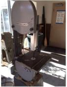
**Design Function** A band saw has a long, thin blade that travels in a constant path around wheels, and pulleys. The only portion of the blade exposed is the area from the table to the top of the work piece. The wheels, pulleys, belts, and all non-working parts of the blade are encased within the machine. The upper guide of a band saw should be set at a height just above the work piece. The intended use is for:
