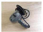
**Design Function:** Disc sanders are used mostly to shape wood as opposed to smoothing it. They can be invaluable fairing tools, though careless use will cause notches and hollows.
