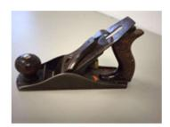
**Bench planes** come in several sizes, the most common of which, by far, is the #4. They are used for general smoothing of stock. Larger bench planes, known as "jointer planes" are used to straighten and flatten stock. They are generally used when a straight, flat surface is required on a piece that is too large to be run across a jointer (see "power tools").
