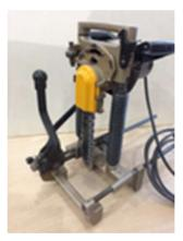
**Design Function:** A chain mortiser, as the name implies, is used to cut mortises in heavy timbers. It can be used to produce a finished mortise although if particularly high-quality work is called for some hand finishing with a chisel may be necessary.
