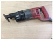
**Design Function:** Fast, rough cuts in wood and metal. Great tool for demolition. This is generally not a precision tool though we have successfully used them to cut the notches in pole rafters.
