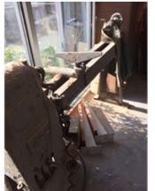
**Design Function:** A lathe works to shape a piece of wood by rotating the stock against a stationary cutting tool. The work piece must be securely clamped between the lathe centers. The tool must be firmly supported on a tool rest, so it will not be thrown towards the operator. The tool rest should be adjusted so that it is 1/8 inch from the largest work piece diameter. If a stationary tailstock center is used it should be oiled or waxed. Intended use is for:
