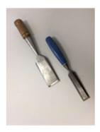
**Paring Chisels** are relatively light chisels, generally used for finer work. Mostly they are pushed by hand, though from time to time it may be useful to tap one with a mallet.
