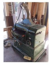
**Design Function:** The cutter head on this equipment rotates at high speed while the work piece is moved beneath it. Straight or segmented knives are mounted in the cutter head.
