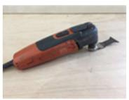
**Design Function:** These are, as the name implies, multipurpose tools. Their main uses are in making small cuts and for sanding into inside corners. I have found that they work very well as a sort of an electric chisel. They are primarily used on wood although we have used them to cut fasteners that couldn't be dealt with any other way.
