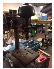
**Design Function:** Drill presses are equipped with rotating chucks that hold drills or other cutting tools (boring bars for instance). Guards are used to prevent operators from reaching into the areas where there
