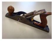
**Rebate planes** are designed to allow cutting right up to an inside corner. They are available in several types and sizes. The most common ones, for cabinet and furniture work, are about 1 - 1 1/2 inches wide and made entirely of steel. The other type of rebate plane (pronounced "rabbit" by-the-way) is the bench rebate plane. It is larger, generally about the size of a number 4 or 5 bench plane and is frequently used in timber framing.
