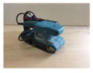
**Design Function:** Belt sanders are used to smooth and to a lesser degree, shape, wood. They can be used, albeit not as effectively, on metal. You will also see them clamped to a horse or a bench top and used as stationary sanders.
