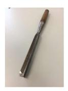
**Corner Chisels** are used almost exclusively to clean up the corners of mortises.
