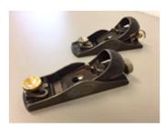
**Block planes** come in two primary types; low angle and standard. The standard block plane is a general use plane small enough to be used effectively with one hand. The low angle block plane is used primarily on end grain. Block planes are suited to relatively rough removal of stock, with the finish work left for the larger "smooth planes".
